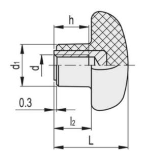
$\begin{array}{lll} D & = 25 \\ D1 & = 12 \\ DH & = M5 \\ h & = 10 \\ I2 & = 10 \\ L & = 20 \\ Weight in (g) = 9 \end{array}$
